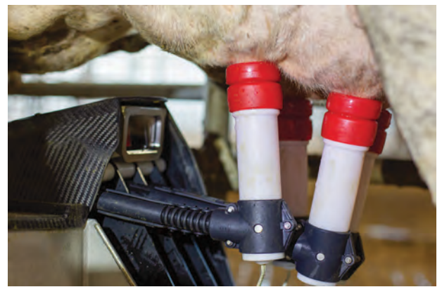
Top photo: As cows are milked, Lauren Collier immediately monitors their health and productivity. Above: Robots use lasers to line up cups and gently milk the cows.
