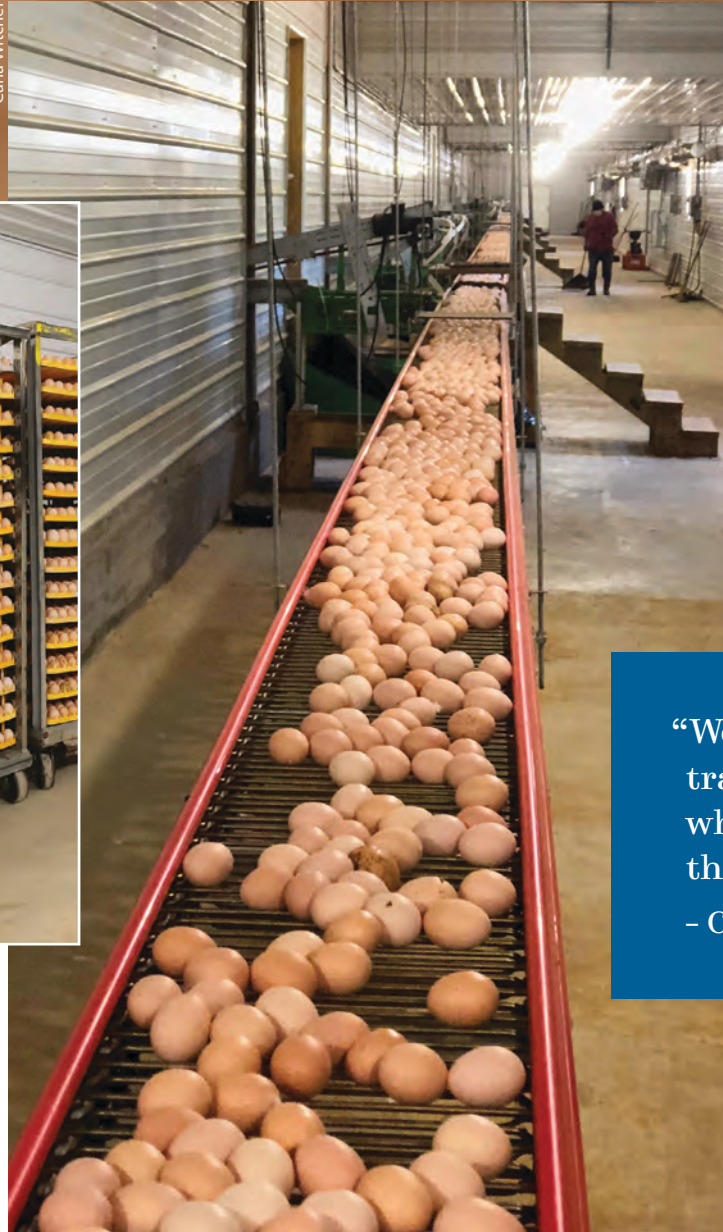
Eggs travel on a conveyor from the nest to a cooler room. There, a robotic picker lifts them off the conveyor and sets them pointed-end down on trays.
